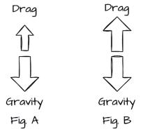
When the parachute first drops (Fig. A), gravity is greater than air resistance, so the parachute falls faster and faster towards the ground. As the parachute keeps going faster and faster, air resistance increases in the opposite direction until it eventually becomes the same in magnitude as gravity (Fig. B). At this point, the parachute reaches terminal velocity, which is the fastest speed reached by the parachute, and it continues to drop at this steady speed for the rest of the way.
